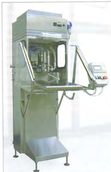
Semiautomatic bottling stations - here the model Liquiwell Filler BIB Italy - pump wines and other still liquids into the pouches. The optimum filling is ensured by inductive metering of the liquids - depending on the capacity of the pouches. (Image source: Liquiwell)
